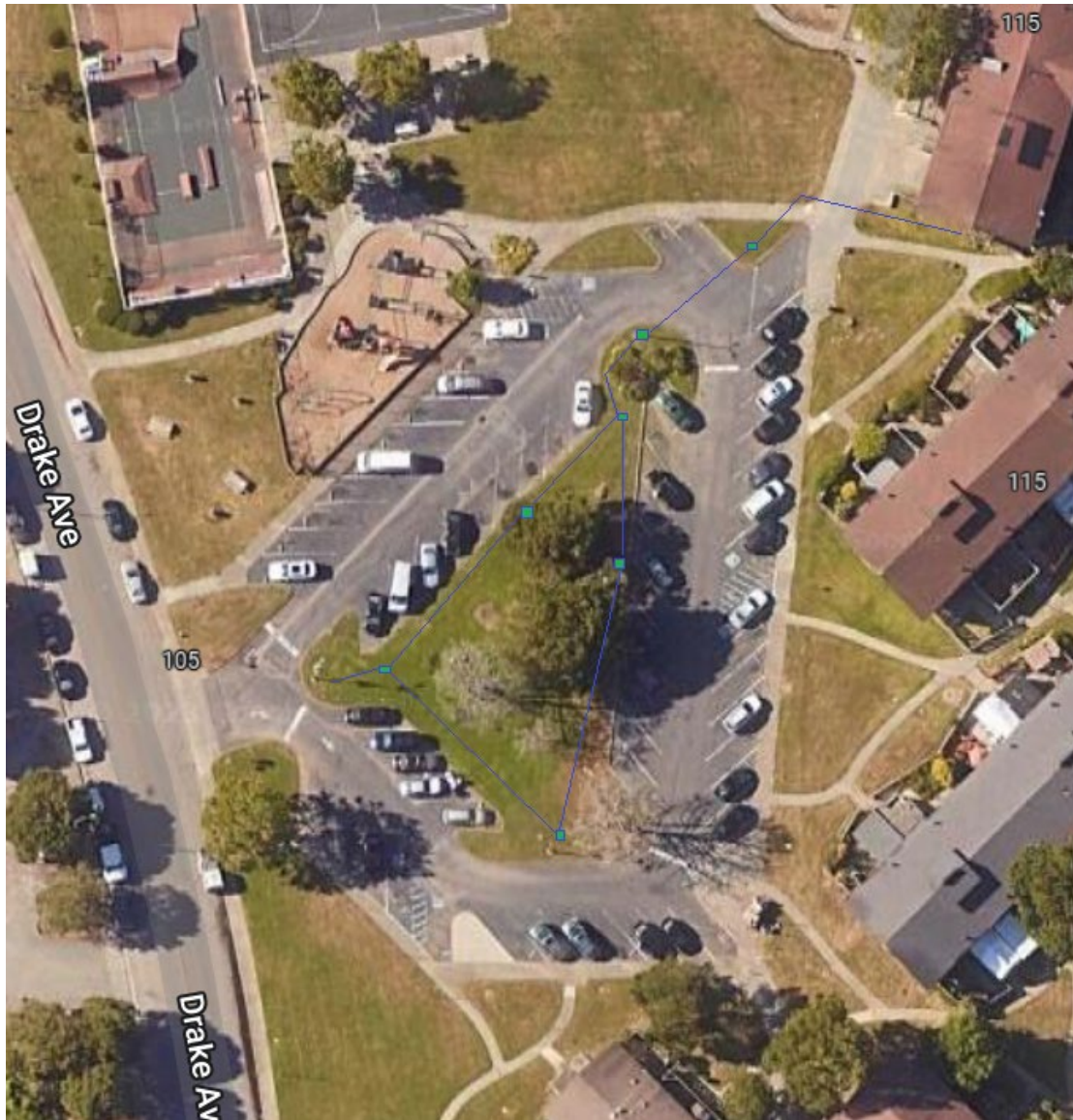
Trenching paths in blue line. Green rectangles represent in ground electrical junction boxes.
