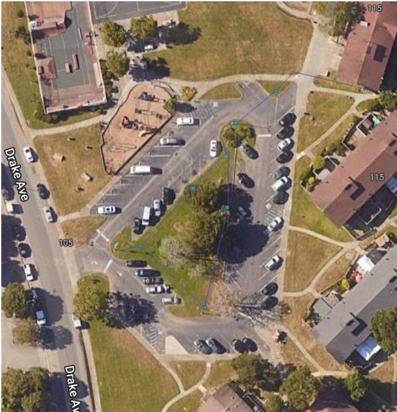
Photo 1 Proposed location and route of trenching for conduit. Building B-12 at top-right, recreational cluster at top-left. Source: MHA, 2023.
