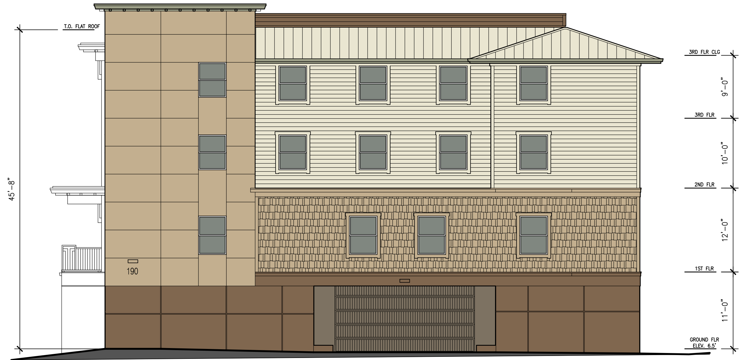
2 SOUTH ELEVATION – MILL ST. A3.2 SCALE: 1/8" = 1'-0"
