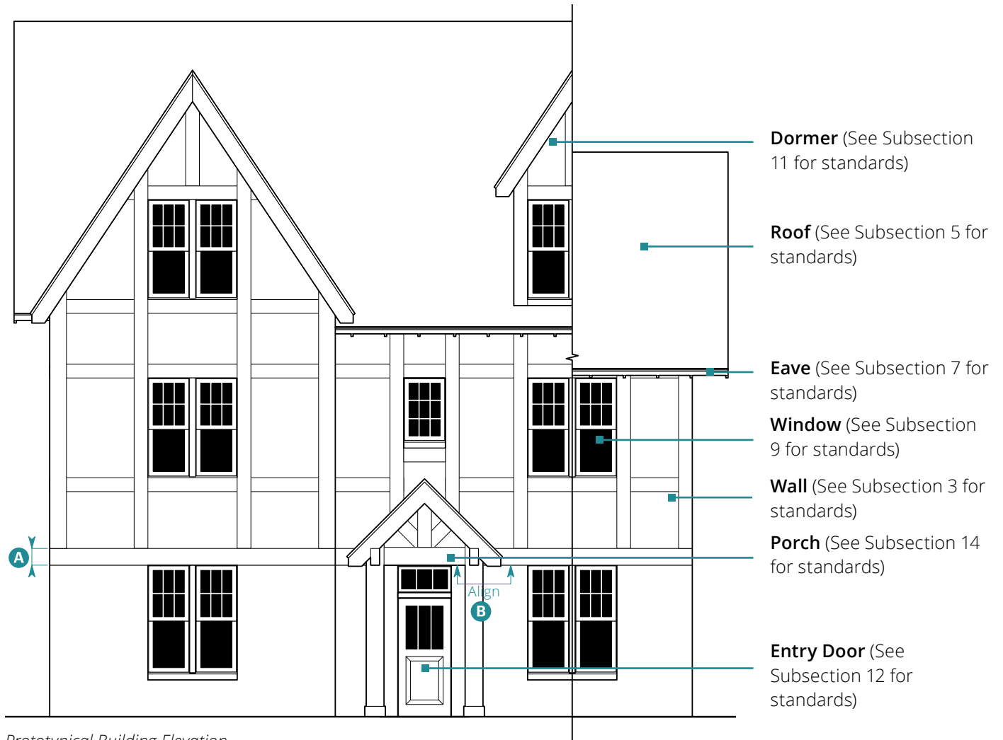
Prototypical Building Elevation
